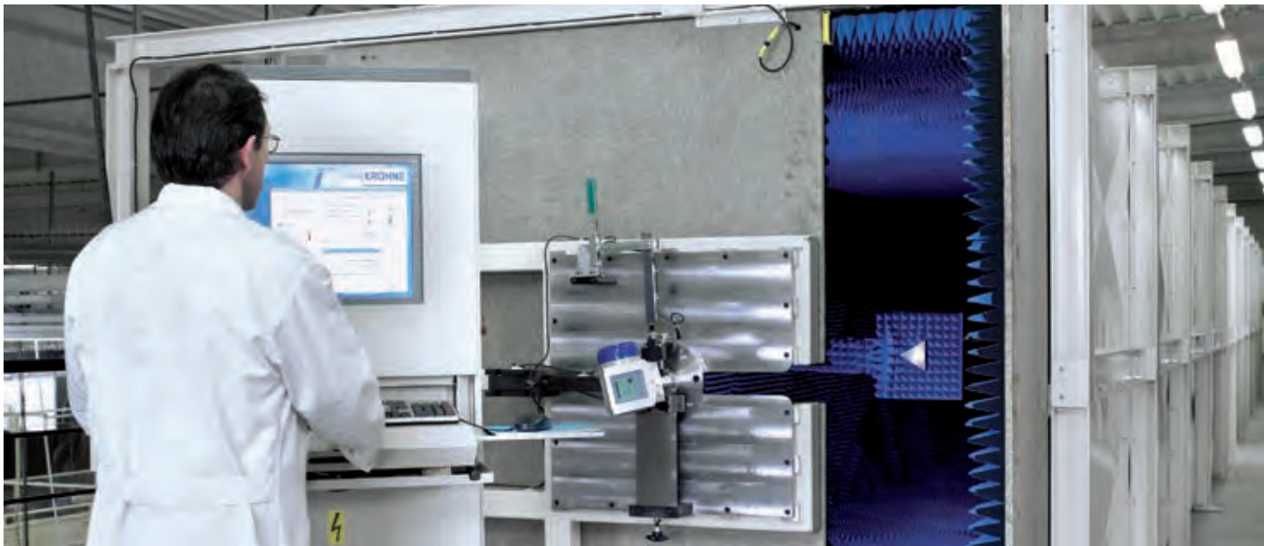
Stretch for calibration of FMCW level transmitters
